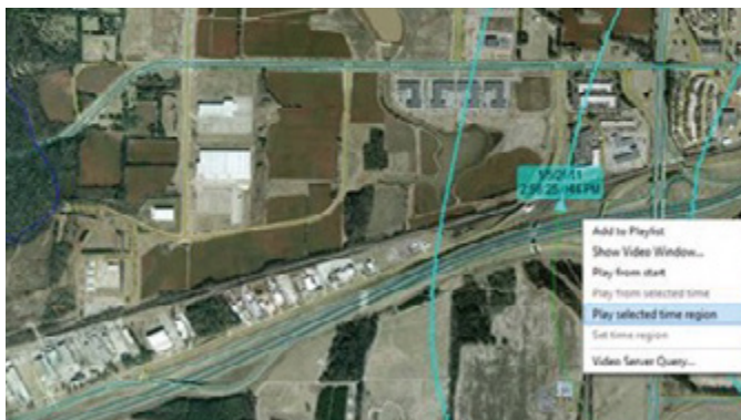
Geospatial vector representations are stored with each full motion video and available for query. You can use the centerline feature to specify what segments of the video to play, as shown here.
