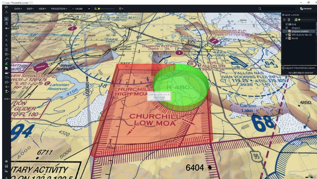
Figure 6 Through a custom Lucy add-on, AIS airspace shapes and constructive geometry operations are combined to create the Churchill Low Military Operations Area (MOA) in Nevada. The MOA consists of a polygonal airspace volume from which a circular airspace volume is subtracted.
