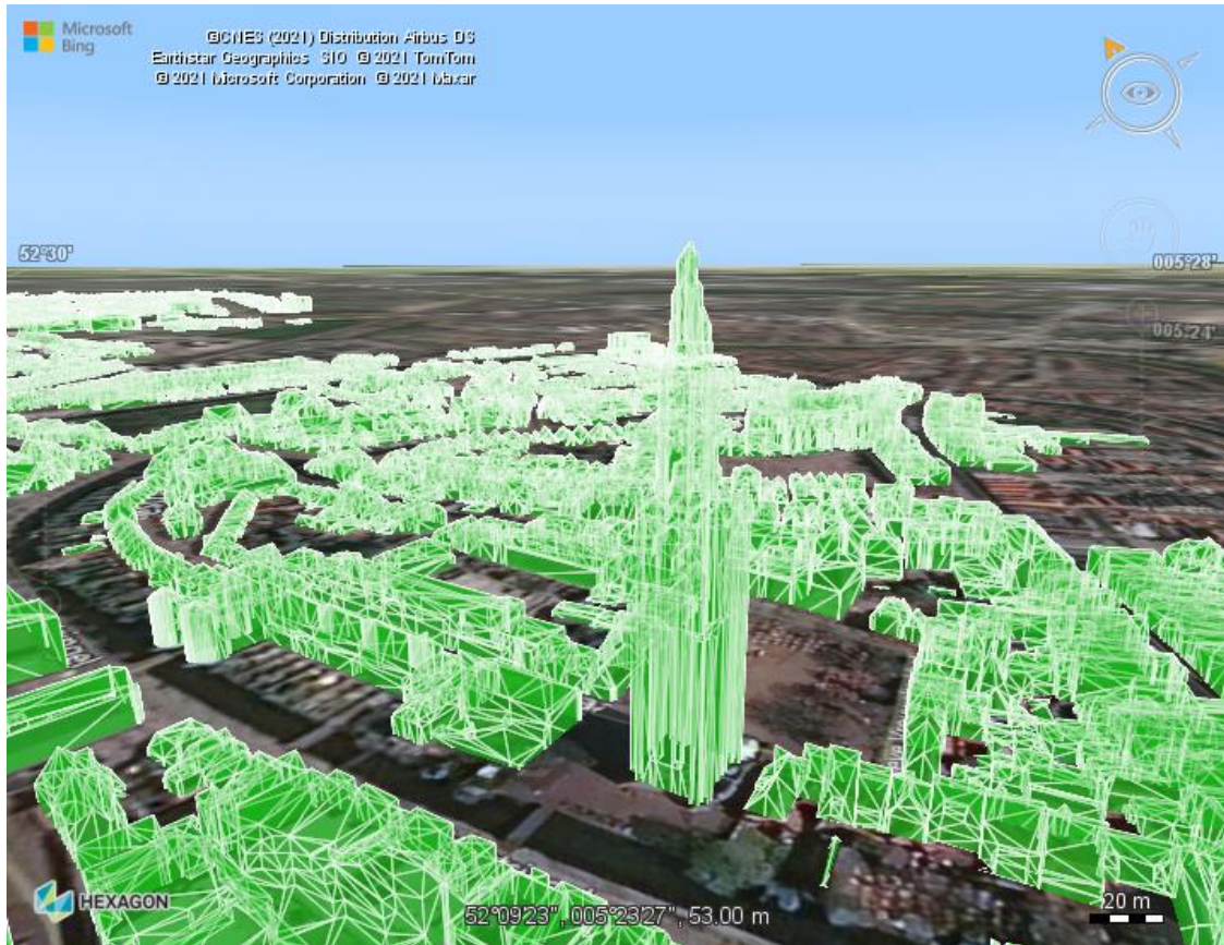
Figure 5: One of the landmarks used for the NAP vertical datum is the church tower in Amersfoort (building data by 3dbag.nl).
